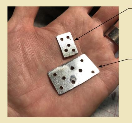
Inner plate / splint, This was created to fit within the cast aluminum frame. The drilled holes allowed for the "cold weld" (J-B Weld) epoxy to "bite" into the splints.
