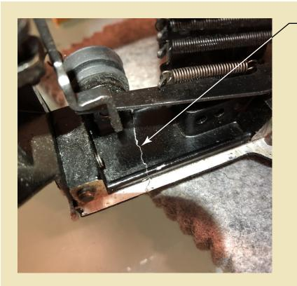
The break was relatively clean and the frame was not bent. A clamp was used to keep tension on the joint. I wanted to splint the inside of the frame before working on the outside splint.
