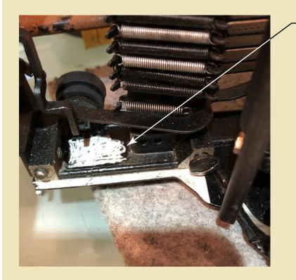
A Dremmel Tool was used to remove the paint so that the weld would have a place to "bite" into. I wanted to get down to the metal instead of gluing to the paint.
