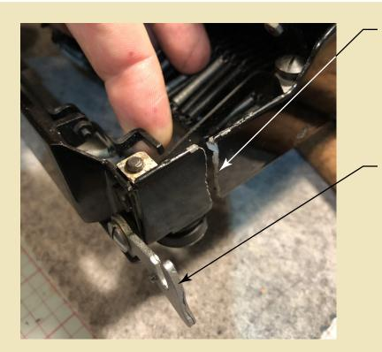
The break was relatively clean and the frame was not bent. The aluminum frame in this area is thin and it makes sense that it would have broken here.
