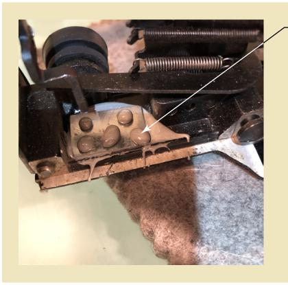
The holes allow for the weld to bite into and go through the plate to grip. The plate was not pushed into the frame at this point.
