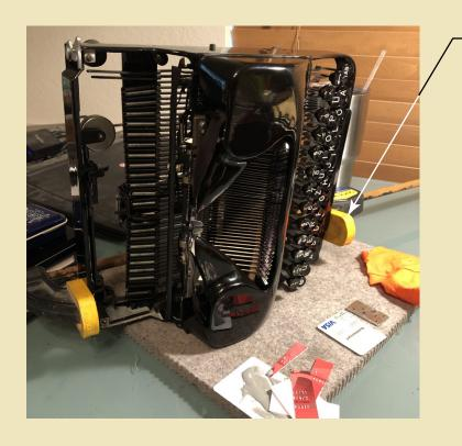
The weld was allowed to cure for 24 hours and the clamp was then removed.
